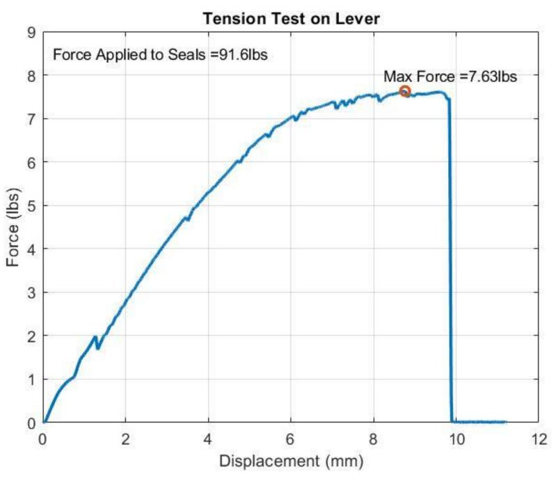
Once the necessary force was known, the strength of the lever and main body was tested to make sure they were strong enough to supply that force. The 3D printed parts were able to supply over double the force needed before delaminating along a layer line. Improvements were then added to the CAD model.
