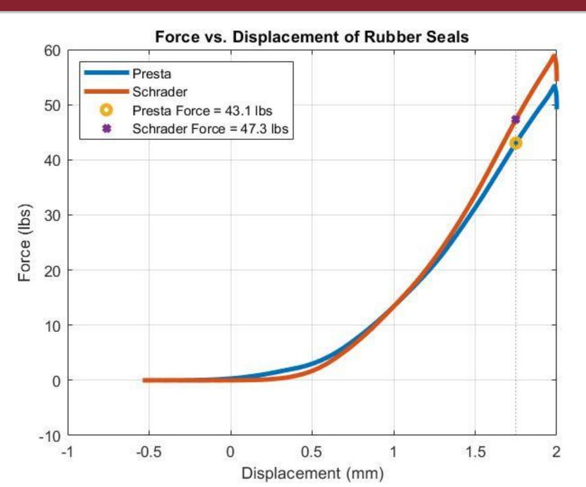
Using the Zwick 5.0 static testing machine, we found that the rubber seals needed about 45lbs of force to compress 1.75mm.
