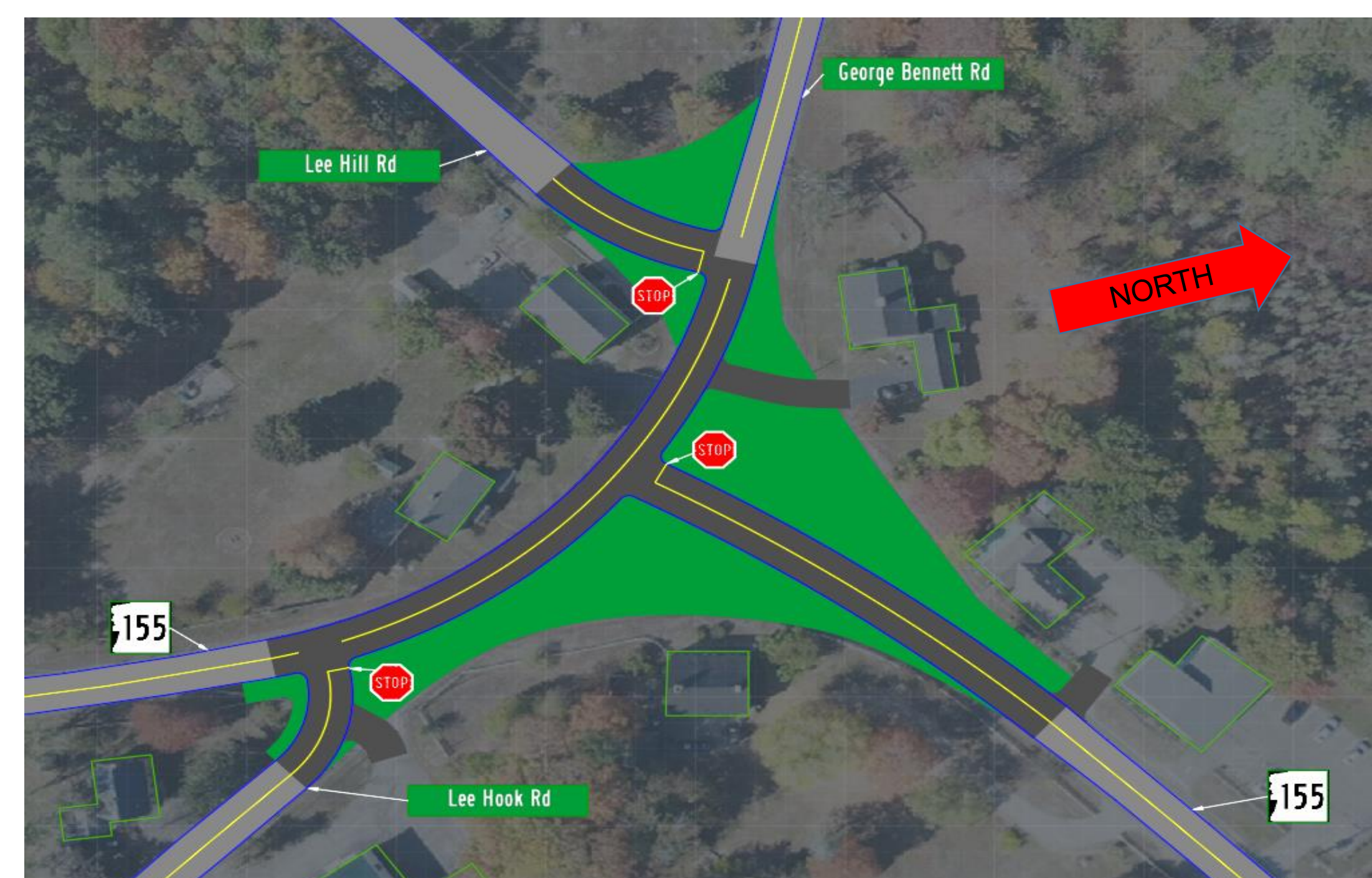
Proposed intersection with re-worked junctions. Design addresses poor sight lines and high speeds on NH 155.
