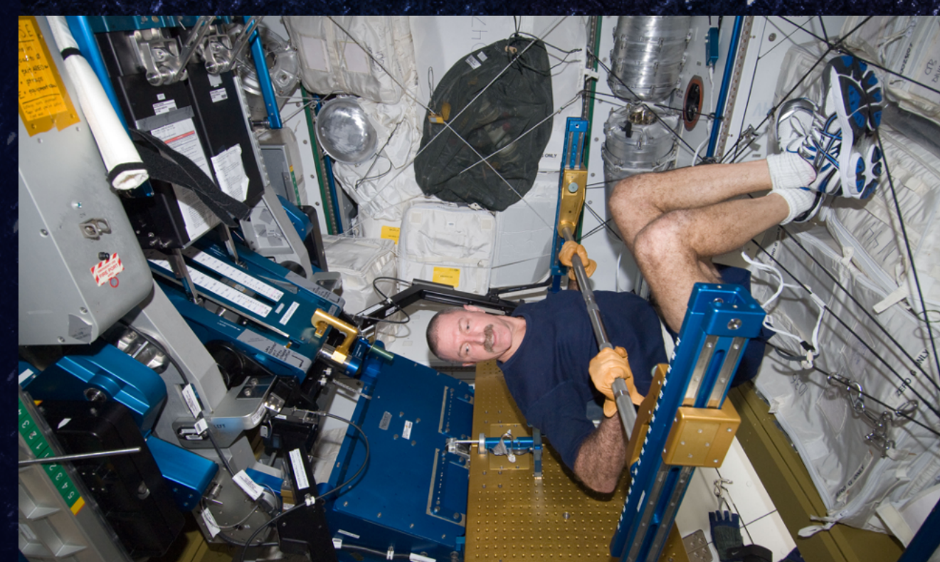
Advanced Resistive Exercise Device (ARED)[5]
