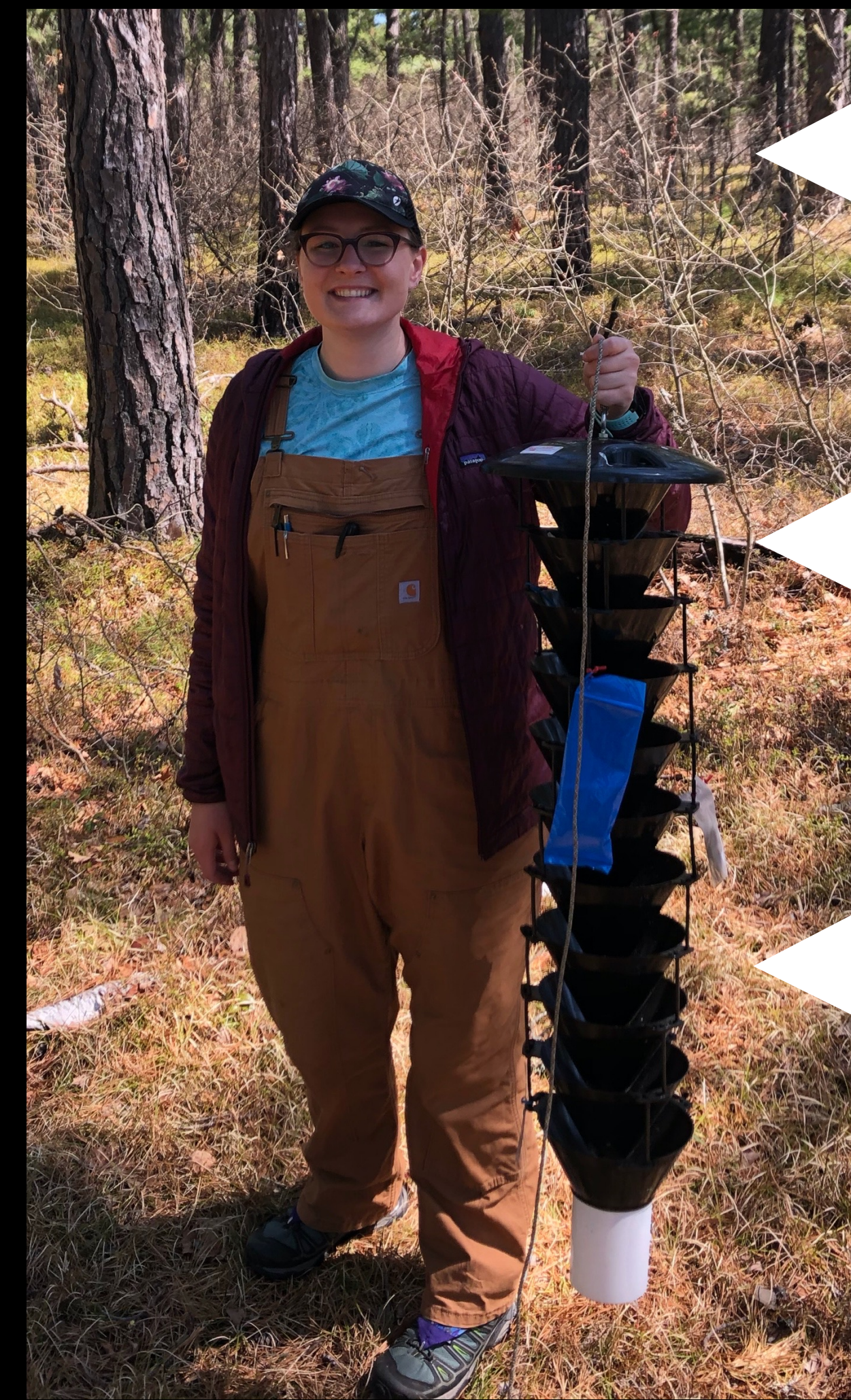
Figure 2. Trapping methods. We deployed 3 Lindgren funnel traps at each site, each with distinct chemical lures.
