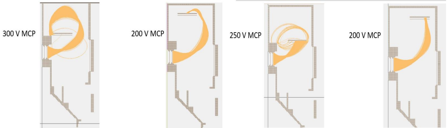
Figure 5: SIMION simulations of curved MCP and anode structure in modified CODIF.
