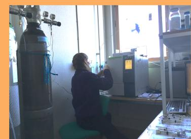
**Figure 5** Gas samples run on a Gas Chromatograph within 24 hours of collection. Photo credit: Clarice Perryman.
