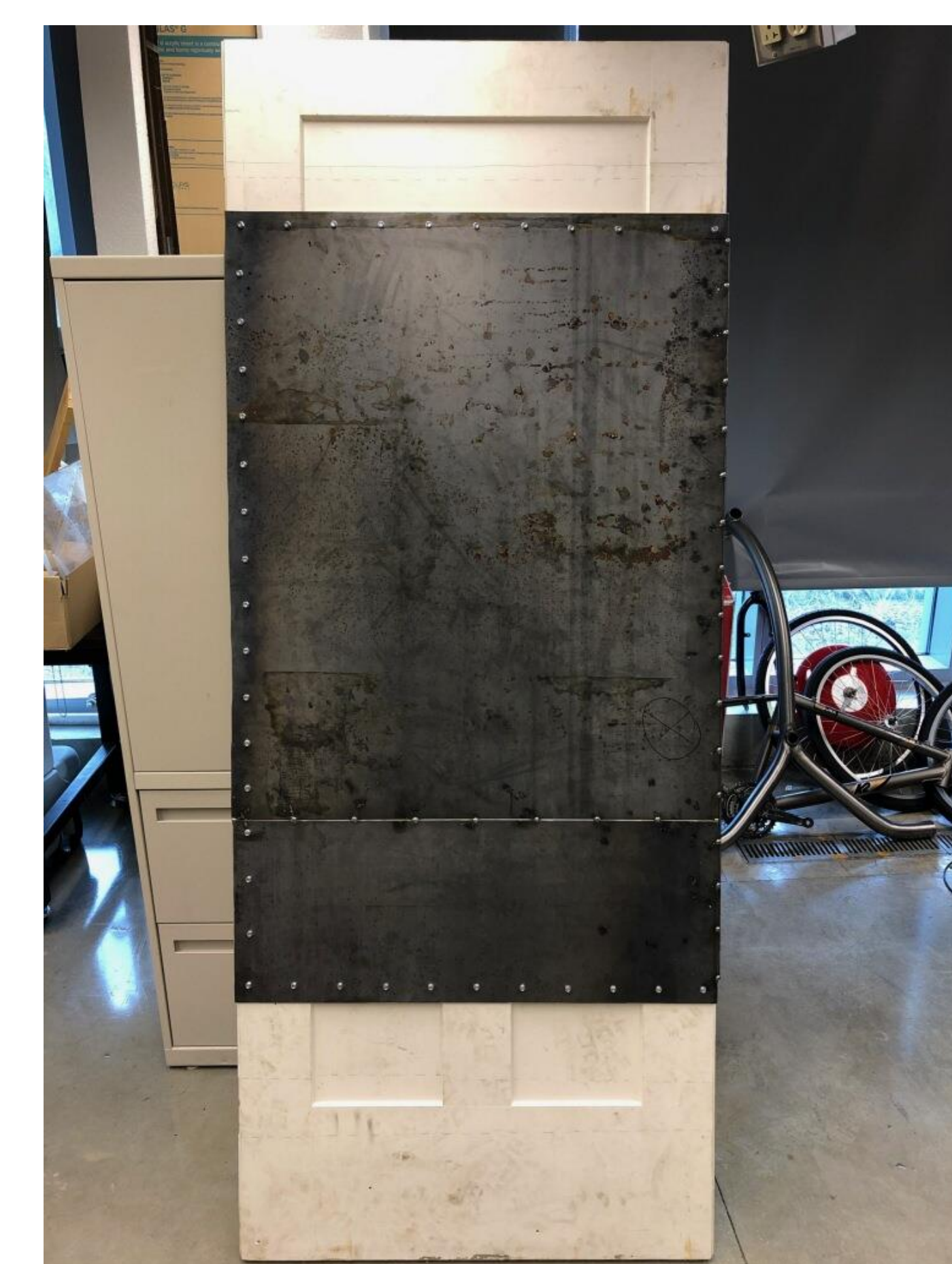
Figure 3: Prototype of door with steel plate.
