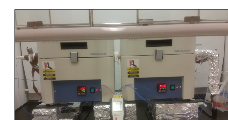
Figure 3 a) Samples underwent Hg extraction via two-stage combustion furnace and subsequent oxidation into a KMnO_4 trap as described in Biswas et al. (2008).
