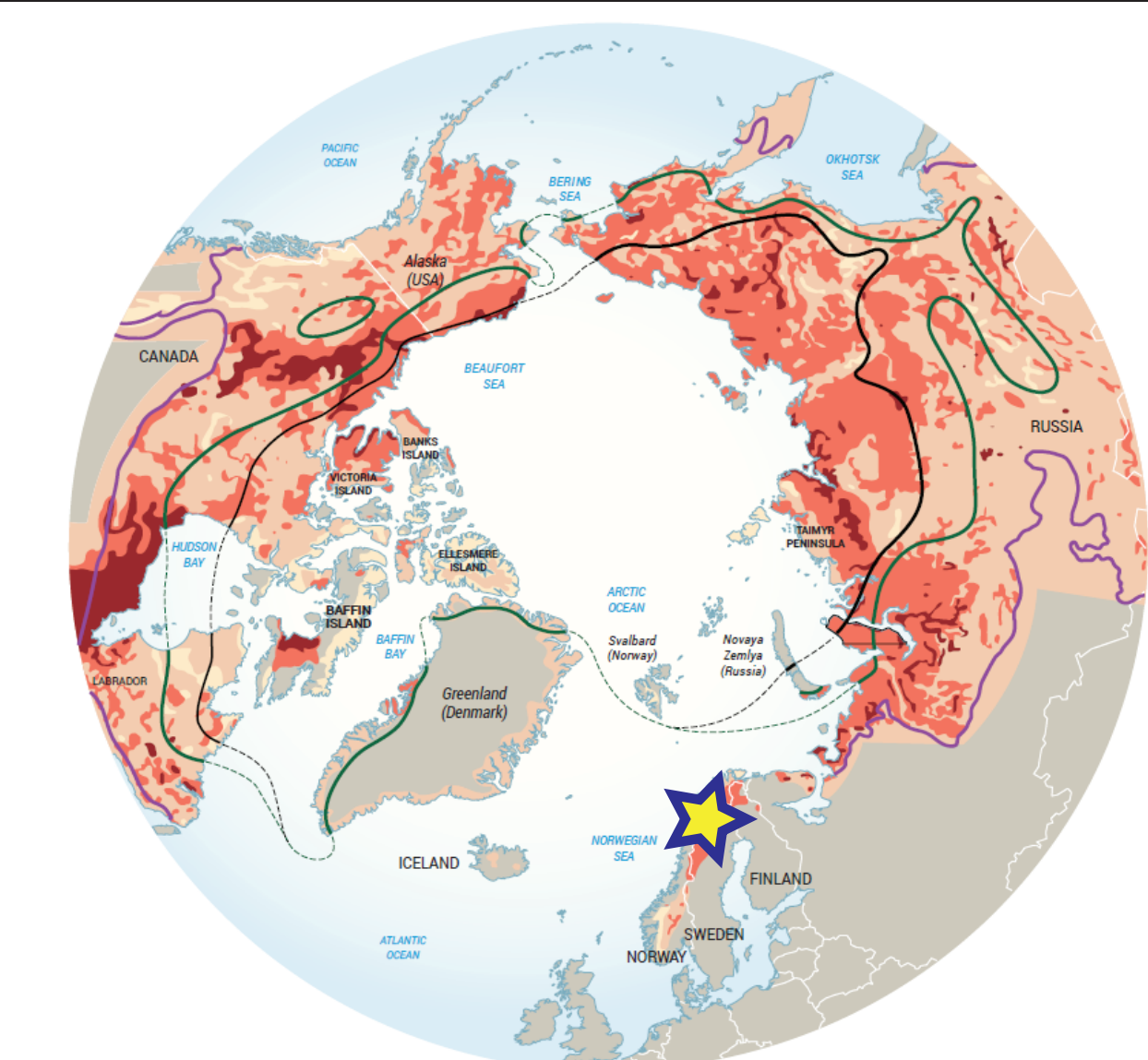
Figure 1. Map of Hg in Arctic soils (Schuster et al., 2018) and permafrost delineations of current and projected (for 2100) permafrost extent, according to Representative Concentrations Pathway (RCP) scenarios 4.5 and 8.5 from IPCC fifth assessment report (Slatyer and Lawrence, 2013; AMAP, 2013). Yellow/blue star denotes study site location.
