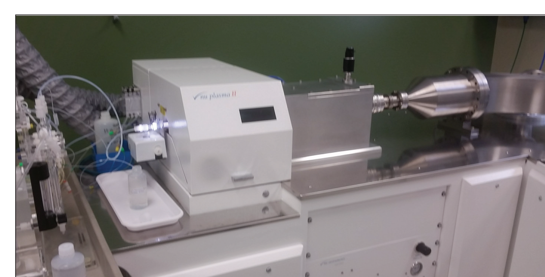
Figure 4. Once extracted and concentrated, Hg is reduced with stannous chloride and introduced via a cold-vapor generation apparatus (CETAC HGX-200) into a nu instruments plasma II.
