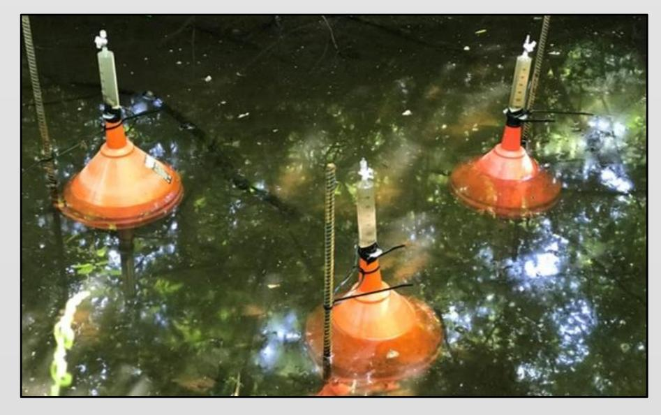
Bubble traps were deployed in triplicate, at four sites within each of four streams of varying land use. Traps were visited weekly from June-October of 2018 and 2018. Captured volume was measured, and some samples were analyzed for gas concentrations. No significant amount of carbon dioxide or nitrous oxide was emitted via ebullition.
