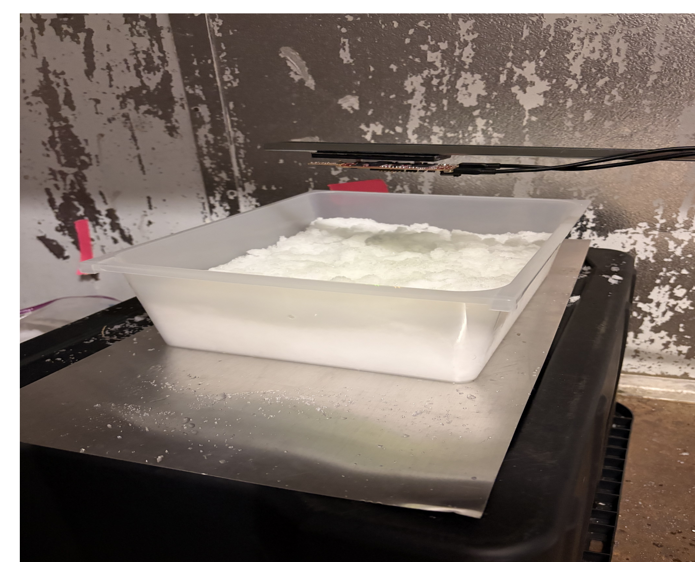
Figure 2: The experimental setup with the radar, snow, and aluminum plate.
