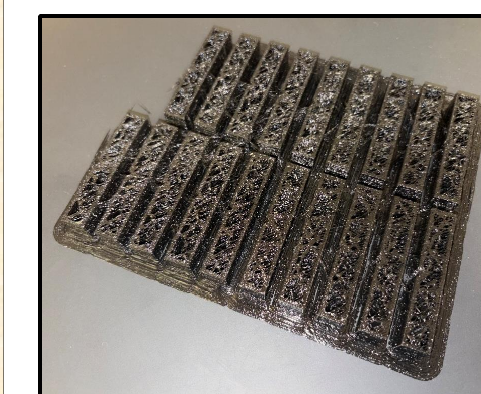
Rough prototype of TPU (flexible 3D printer filament) Izod test specimens
