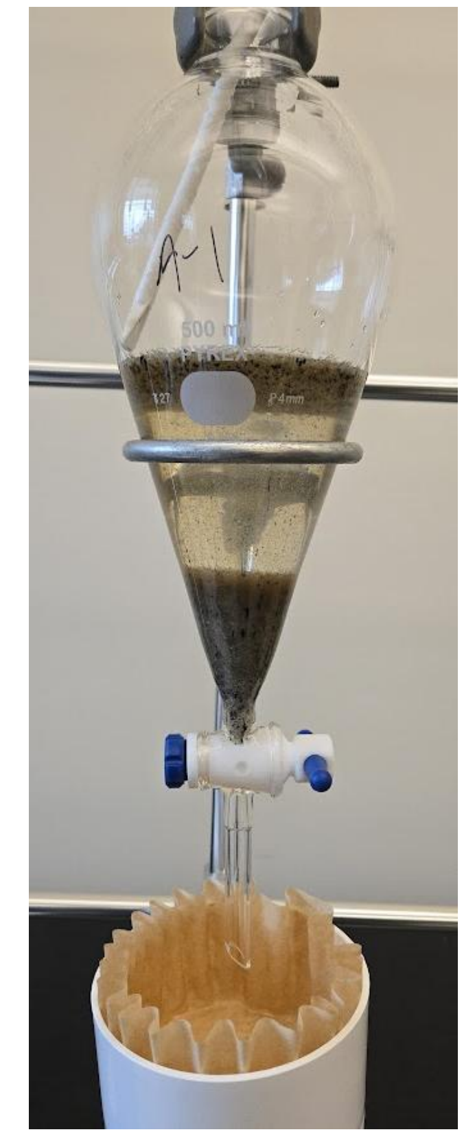
Figure 7. Heavy Liquid Separation
