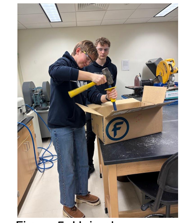
Figure 5. Using hammer and chisel to break down initial sample.
