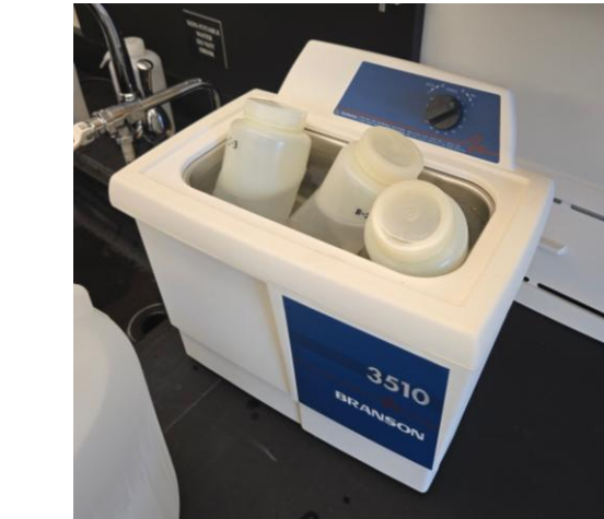
Figure 8. Sonicator vibrates the minerals in water, suspending fine particles.
