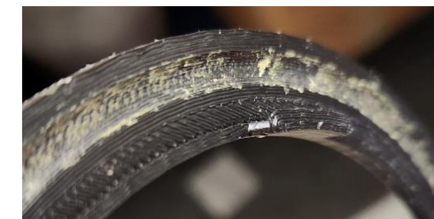
Fig 7: Damaged bearing after continued operation
