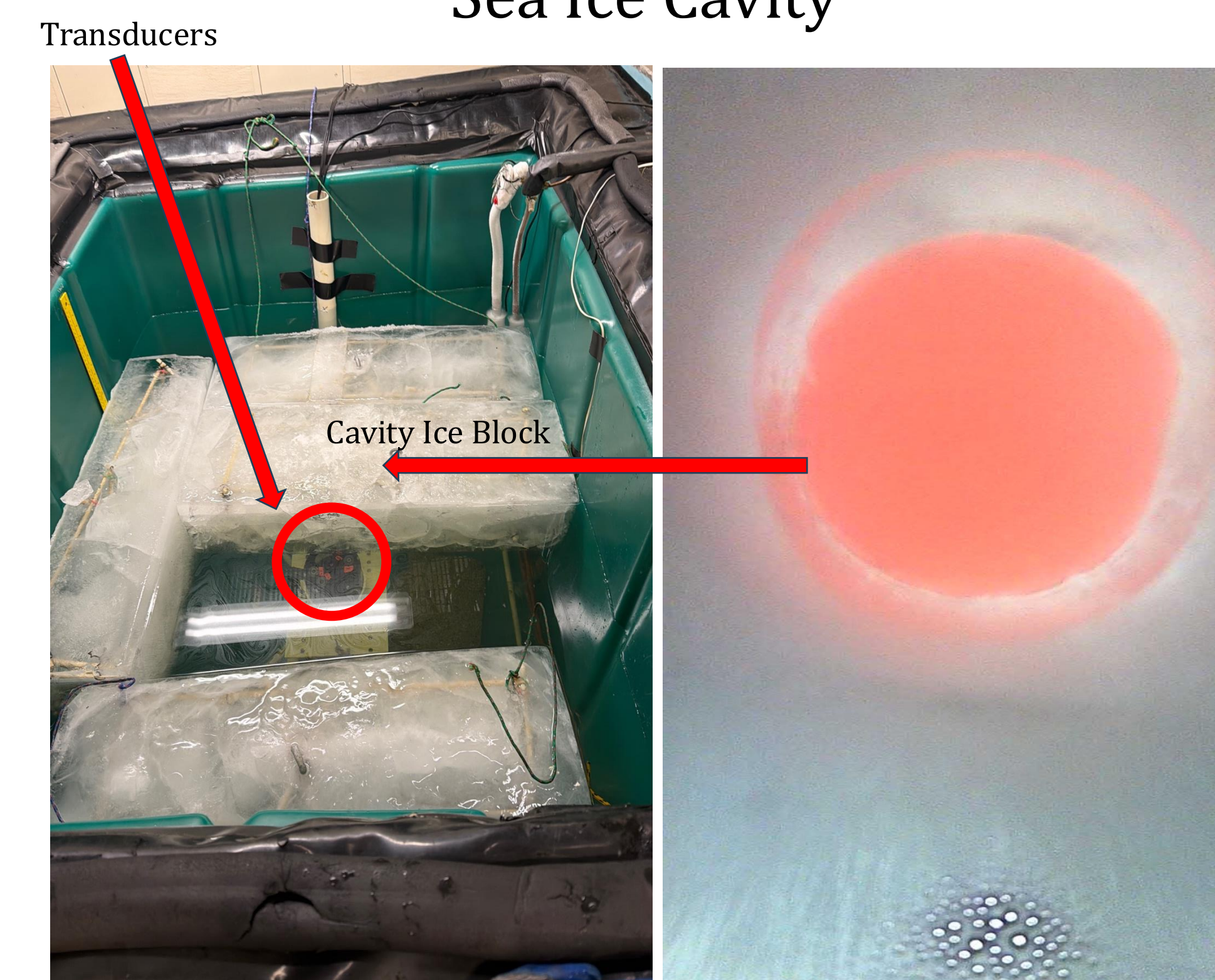
Ice tank with transducers placed in center of tank. Right image is the cavity filled with MD (dyed red) as viewed beneath the ice.
