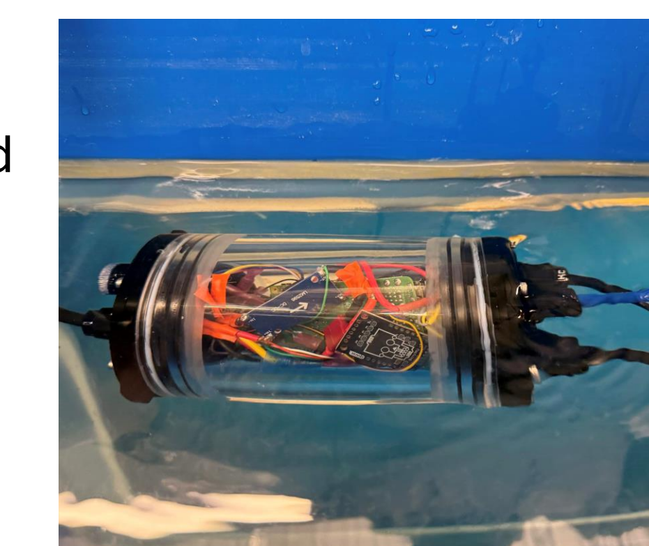
Figure 6: Waterproof Testing of GUPPS Core
