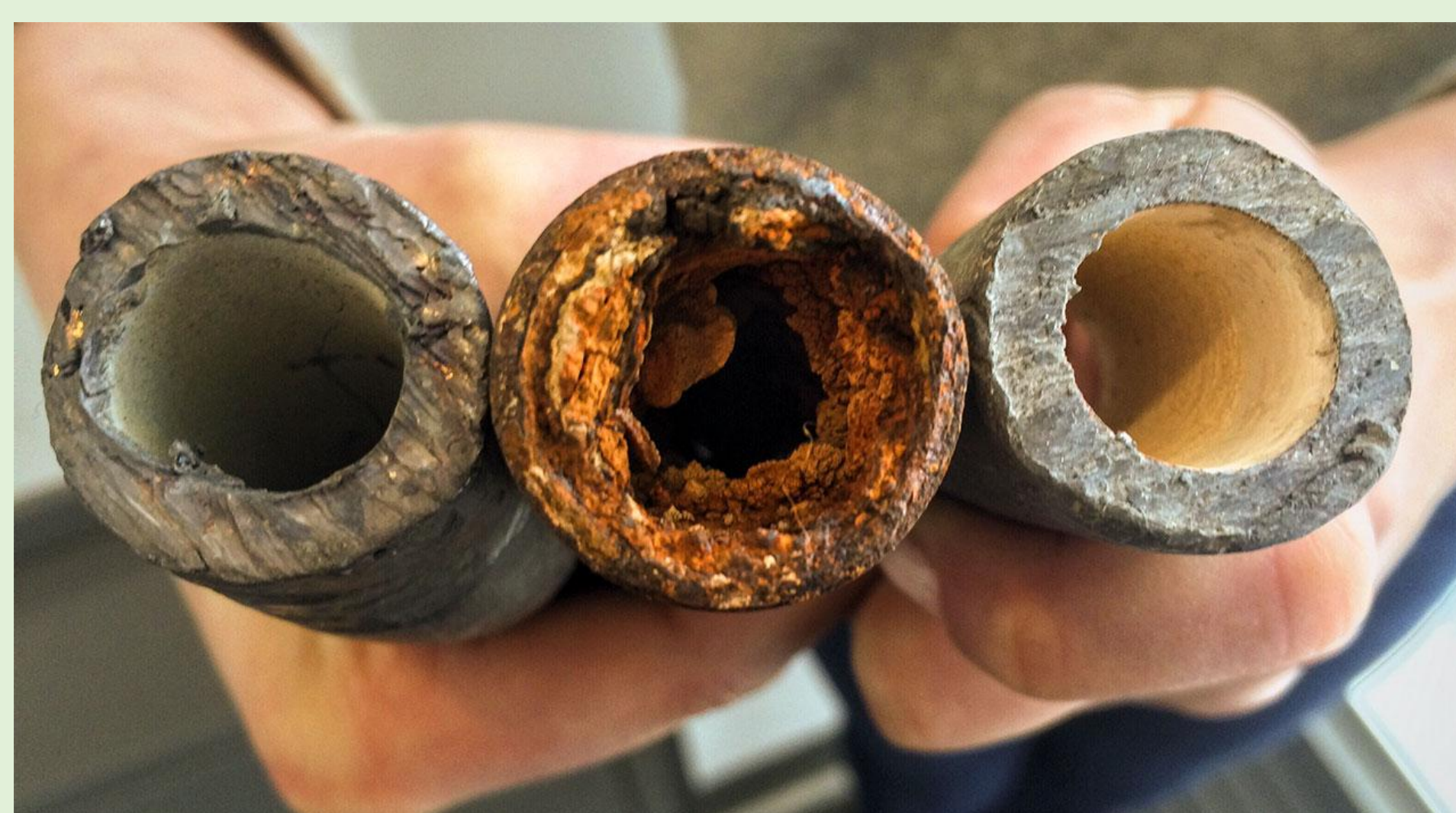
Comparison of new (left), untreated (middle), and orthophosphate treated (right) lead pipes.
