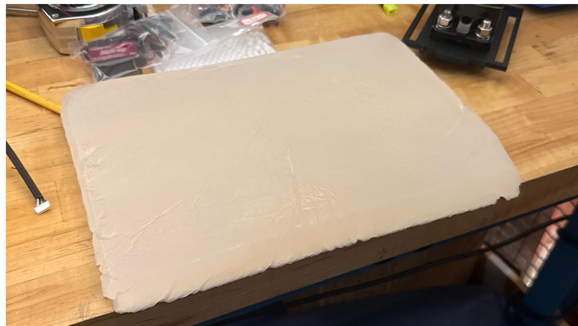
Figure 5: Pictured, is the synthetic whale skin created from rubber, as the base, and epoxy resin layered on top, to allow for realistic testing scenarios.
