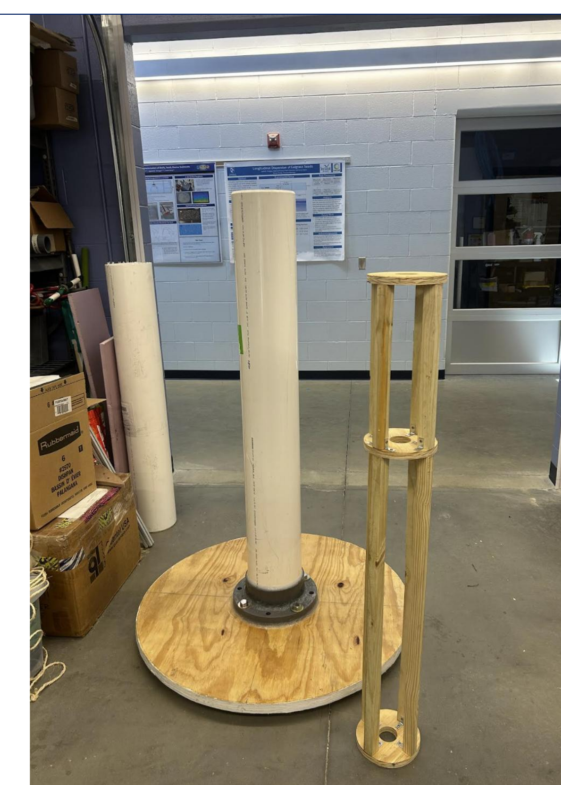
Figure 7: Assembly of Spar and Internal Frame
