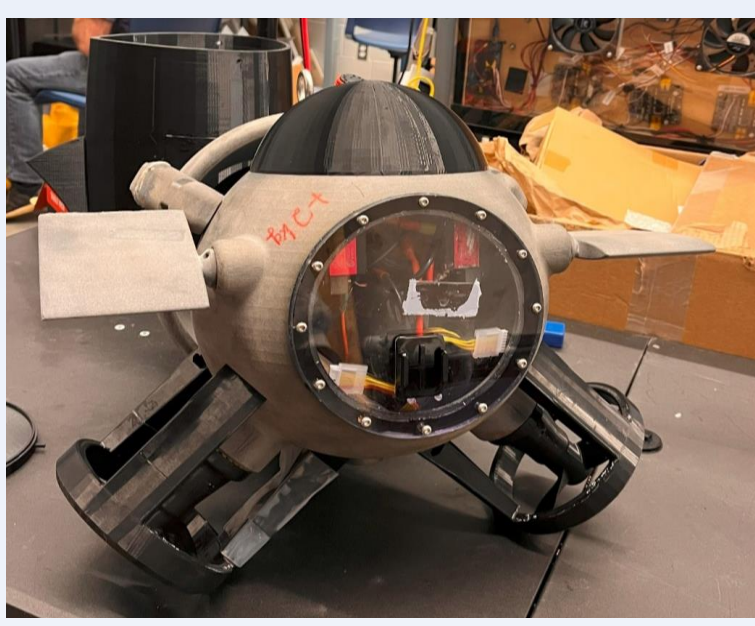
Fig 9: Buoyancy Control Device Mounted on KRILL
