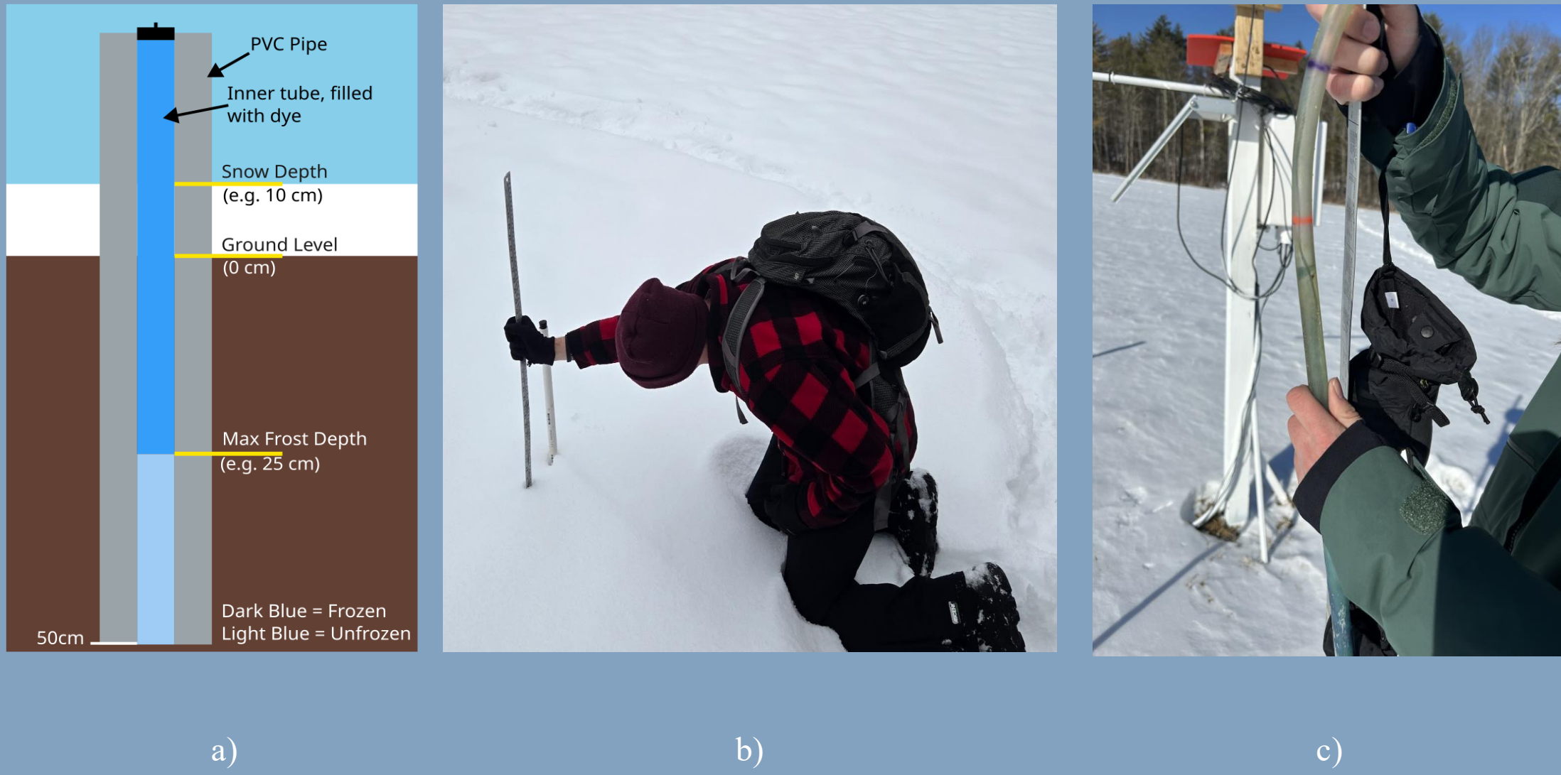
Figure 2. Images of an undergraduate student taking snow (b) and frost samples (c) at a frost tube after a snowstorm. Sampling was performed 2-3 times a week during the 2024-2025 winter. (a) is a labeled diagram of the frost tubes that we used, and the measurements that were taken.
