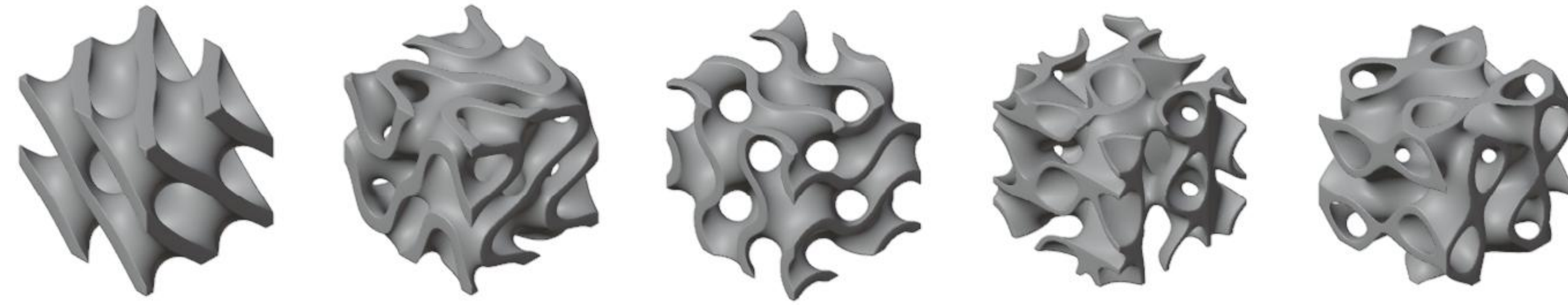
Figure 1: A selection of some TPMSs. From left to right: Diamond, Fischer-Koch S (FKS), Gyroid, Lidinoid, Split-P
