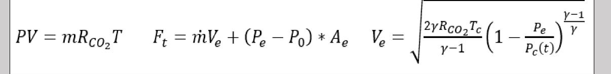
Pressure in Canister as a function of time:
