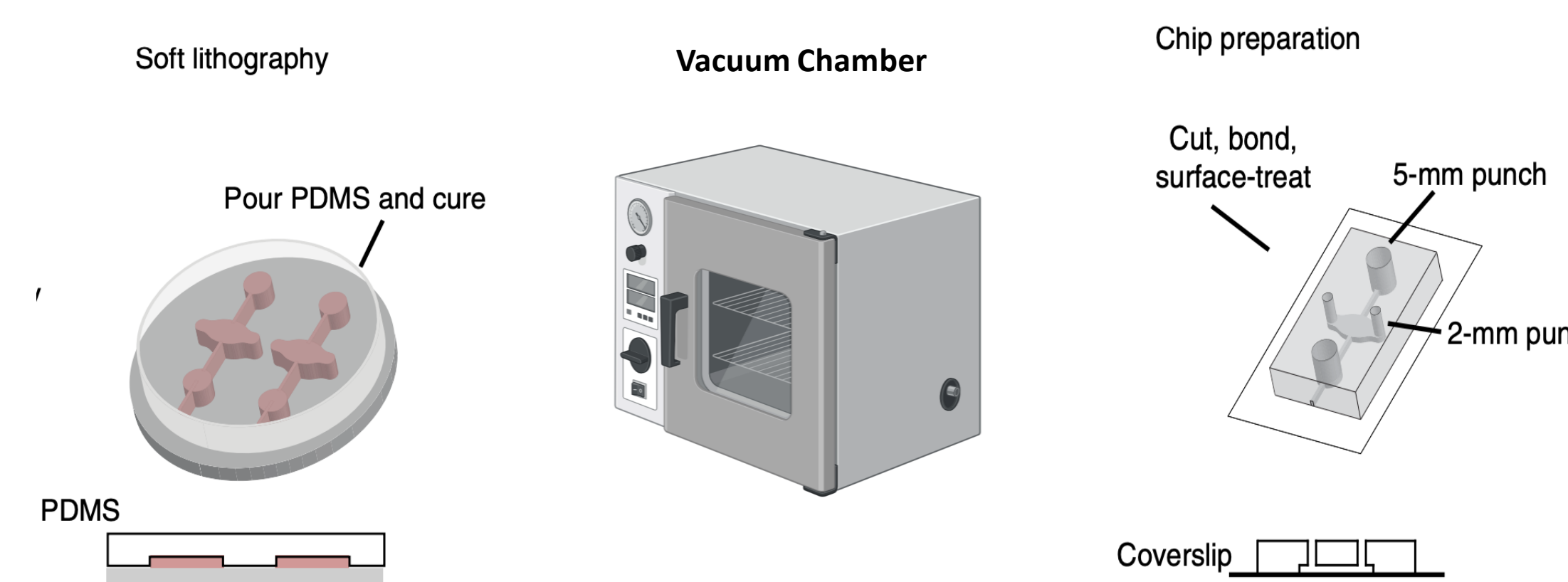
Figure 2. Pouring and curing of PDMS to create chip.
