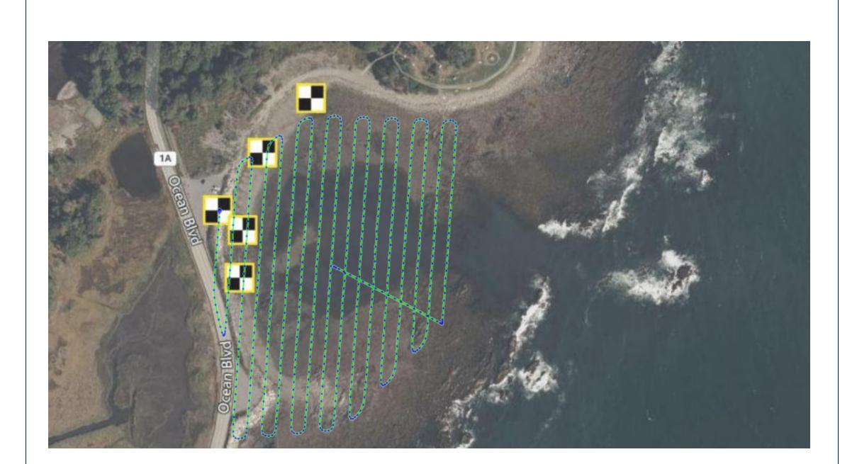
Ground Control Points (GCPs) are compared against Propeller AeroPoint's database to ensure accurate locations.
