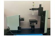
This instrument optically measures the surface tension of a liquid sample using a high zoom camera. Based on the density ( $\rho$ ) of the solution and geometry ( $\beta$ ) of a droplet the surface tension ( $\gamma$ ) is calculated.  $R_0$  describes the radius of the drop at the apex of curvature. The software uses the Young-Laplace method to estimate dimensions of the droplet where  $\beta$  is a combination of 3 equations.<sup>2</sup>
