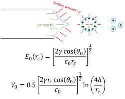
These equations use the dimensions of the emitter tip,  $(\mathbf{r}_{c}, \mathbf{h}, \boldsymbol{\theta}_{0})$  to relate surface tension  $(\boldsymbol{\gamma})$  to the onset voltage  $(\mathbf{V}_{0})$  and electric field  $(\mathbf{E}_{0})$ .<sup>1</sup> The goal of our project was to examine the effects of solutes on surface tension. This work was done using a *Biolin Scientific* ThetaLite 100 tensiometer.
