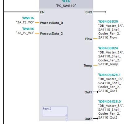
In Main OB1, the function call blocks were added for each of the 83 sensors. This is where the data change from tag to type occurs.
