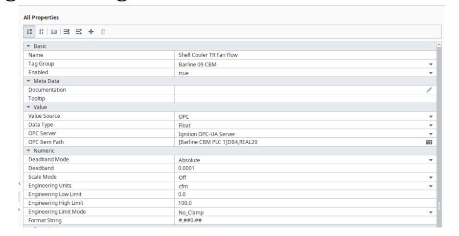
Tags were constructed to pull the output data from the PLC into Ignition for centralized data and analysis.
