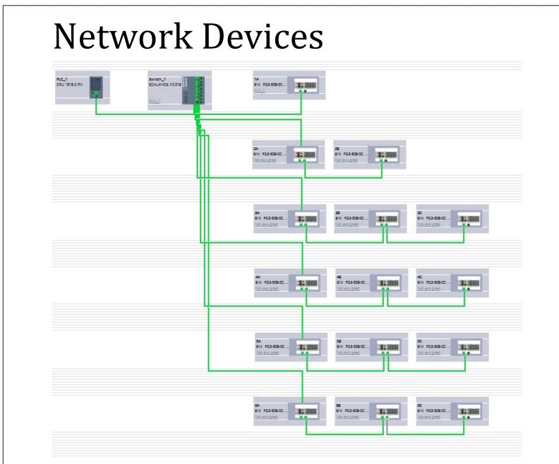
The PLC, switch, and 15 IO Link Masters were added and connected according to the connection charts.
