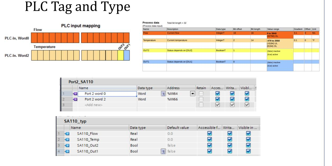
The user manuals were used to set up 83 tags and 7 types in the Siemens TIA Portal PLC programming software.
