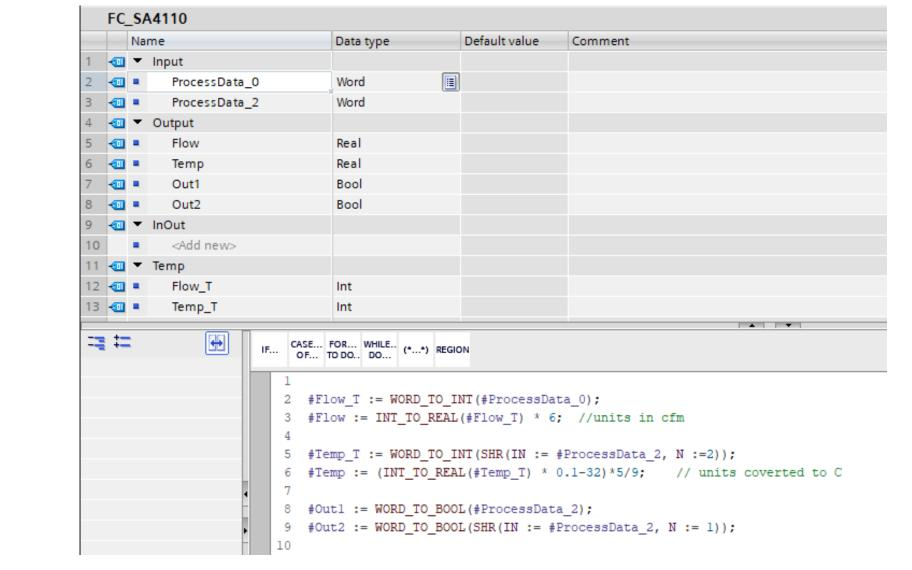
The function calls take the words that come into the PLC and separates them into the desired parameters.
