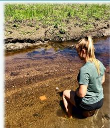
Figure 6. Example of a submerged aquatic ground control point
