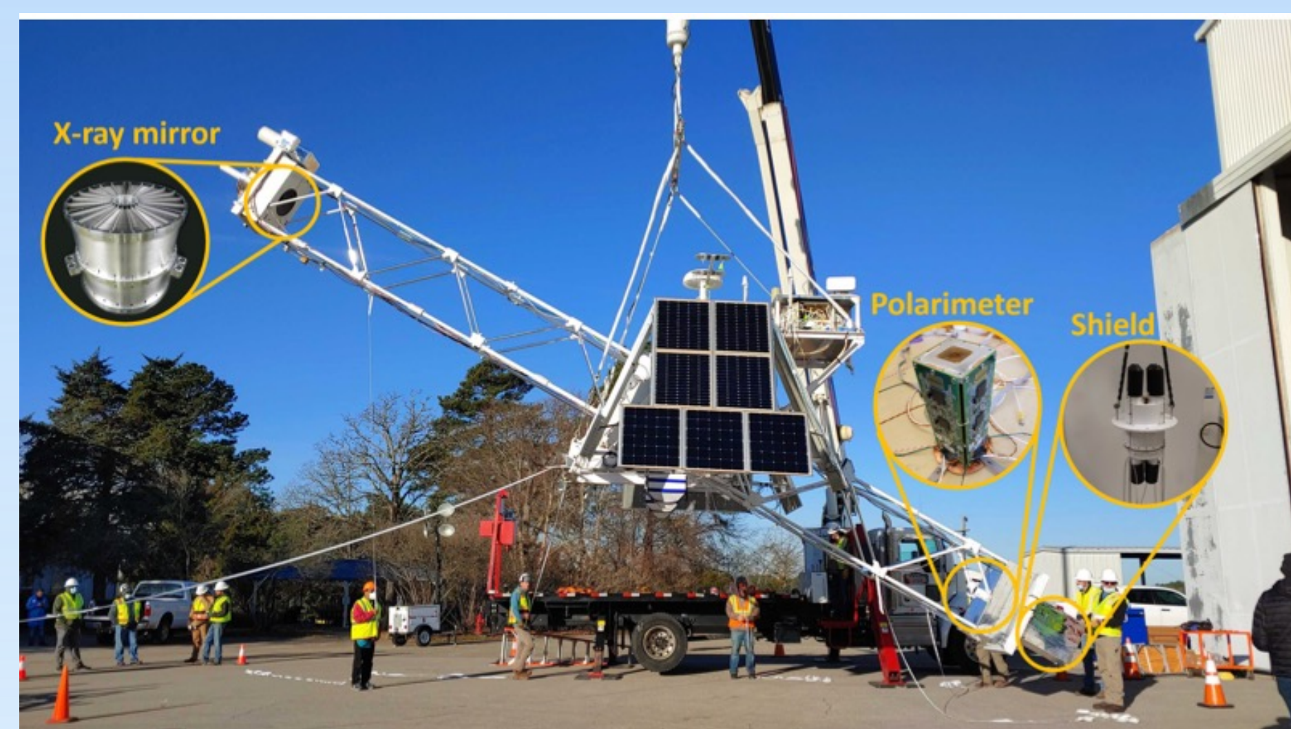
[Figure 1]: XL-Calibur, highlighting the X-ray mirror, polarimeter, and shield. [1]
