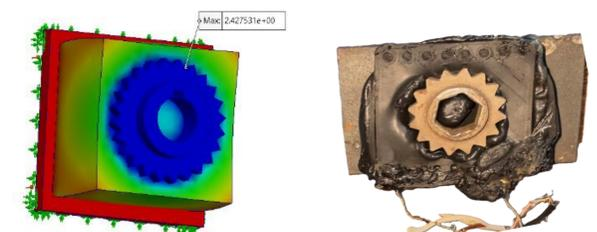
Comparison of experimental test with simulation
