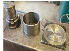
Mold used for heated compression
