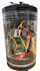
Fig 7. Waterproof enclosure and internal wiring
