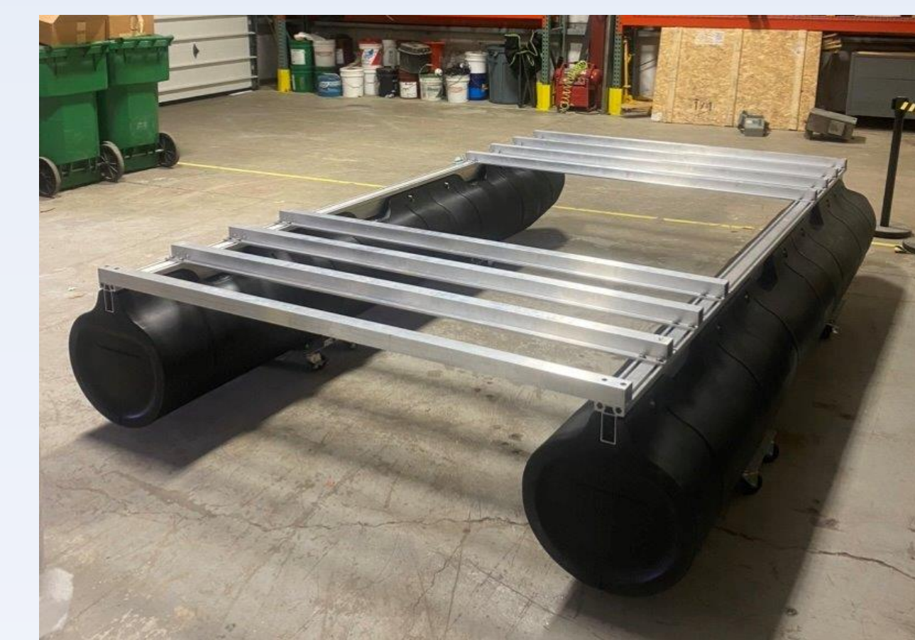
Figure 5: Constructed pontoons with base framing
