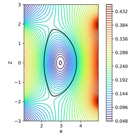
Figure 5. A free-boundary solution with an Ohmic heating solenoid and two poloidal field coils located outside of the computational boundary.
