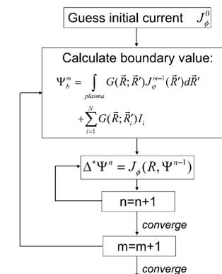
Figure 4. A flowchart showing the code's nested loop structure.
