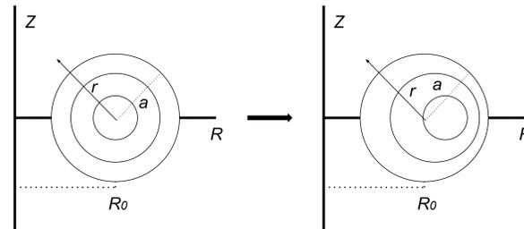
Figure 2. A diagram of how the flux surfaces of constant  $\psi$  are shifted outward as a result of the Shafranov shift. Note that  $\bar{r}$ ,  $a$ , and  $R_0$  are from the center of the outer most flux surface, and not necessarily from the magnetic axis.
