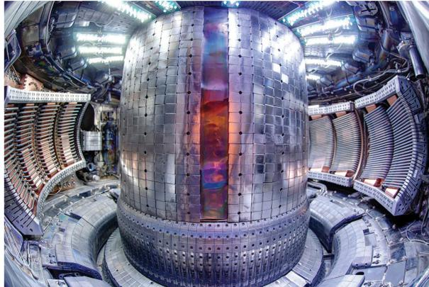
Figure 1. A photo of the interior of Alcator C-Mod, a small, decommissioned tokamak that holds the record for largest average plasma pressure at 2.05 atmospheres.
