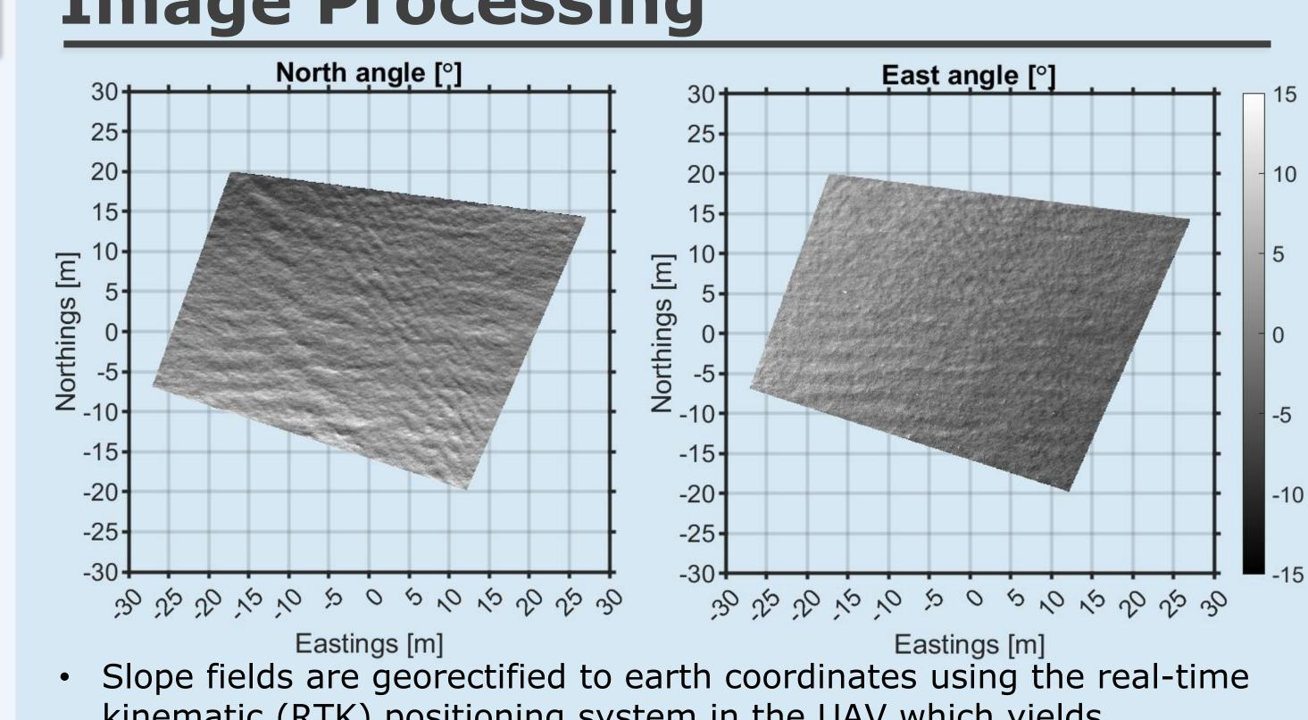
kinematic (RTK) positioning system in the UAV which yields centimeter-scale accuracy.
