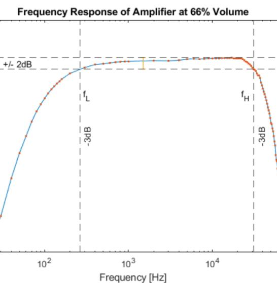
The frequency response of the amplifier has a passband of 260Hz - 31kHz. The amplifier has a maximum voltage gain of approximately 114 with an output magnitude of 41dB.
