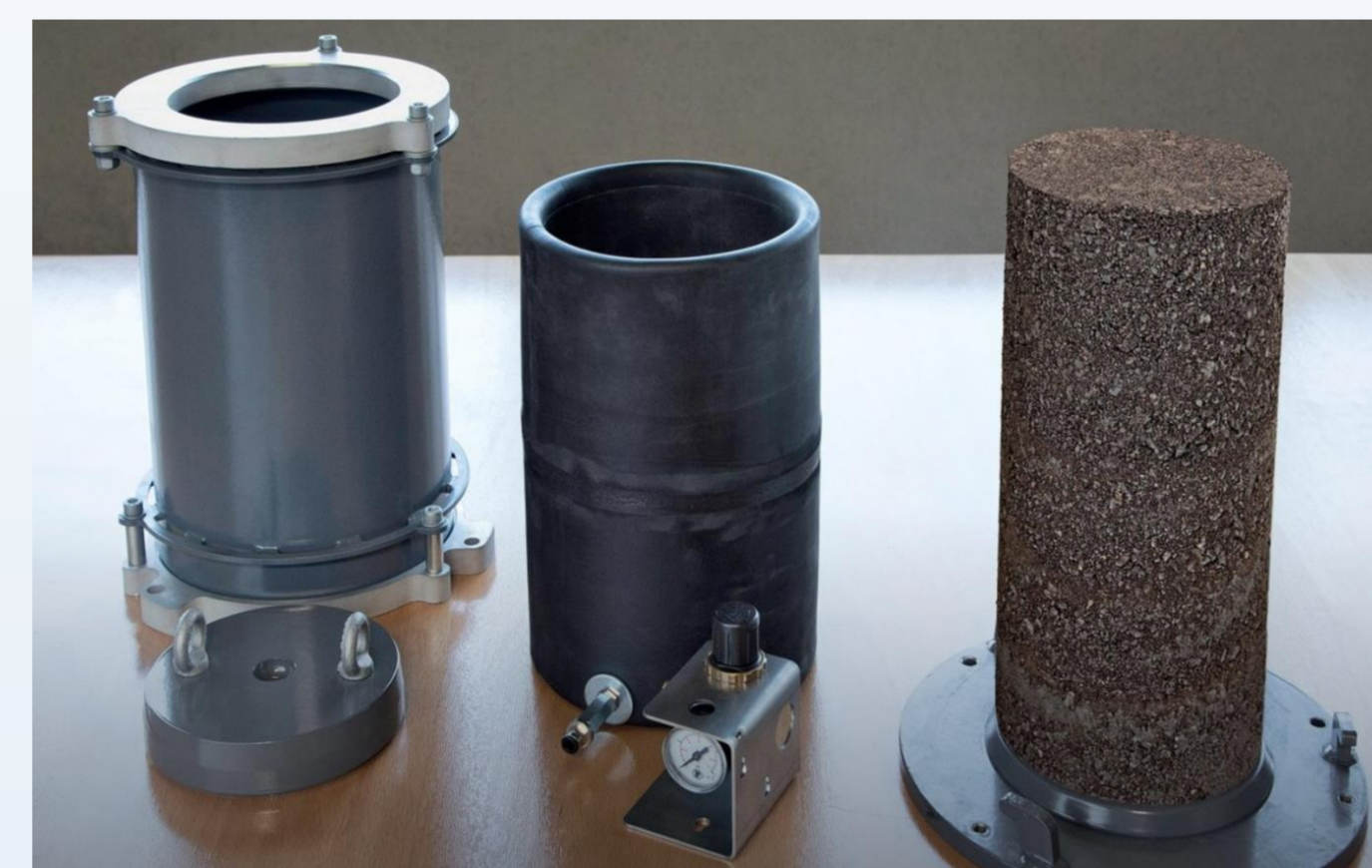
3) Final specimens: 150 mm diameter and 300 mm height.
