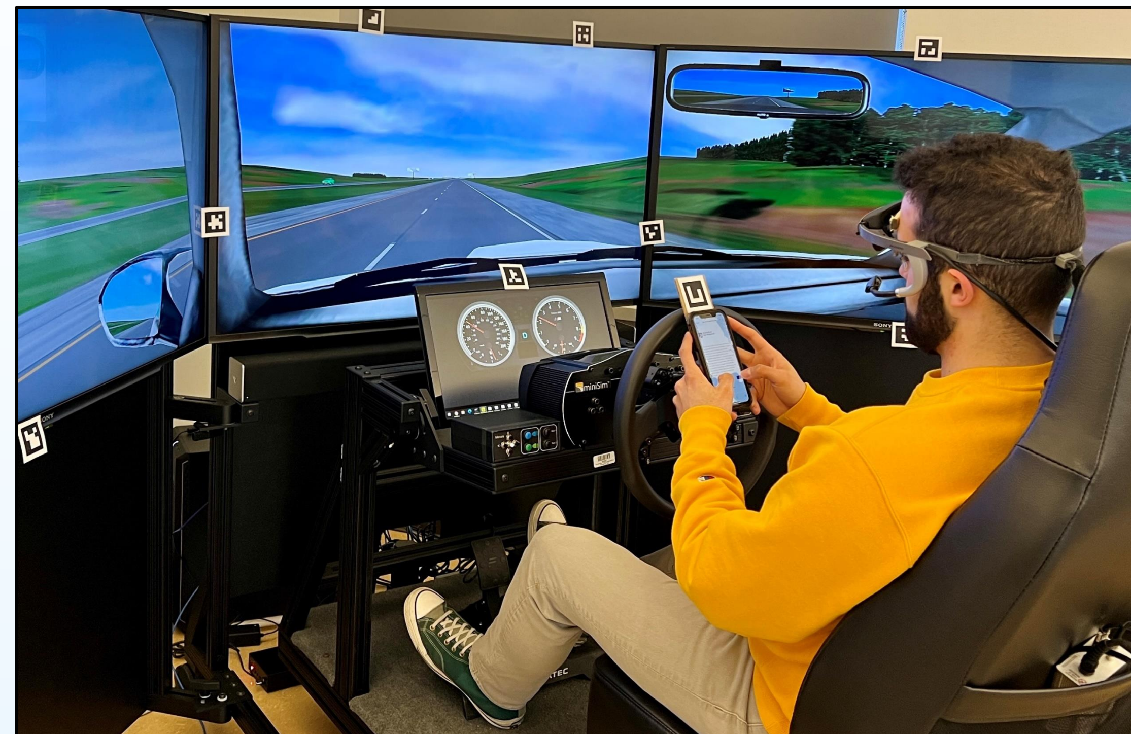
Figure 4: Participant Wearing Eye-Tracker and Texting During Automated Driving
