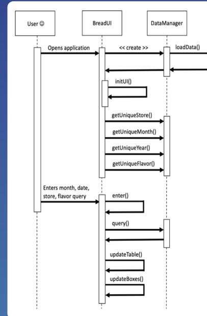
Figure 1: A UML Sequence Diagram Showing the flow of execution for a user query
