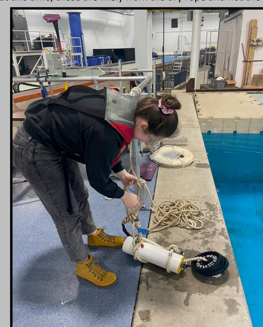
Image 5: Anne securing the instrument with weights and ropes to drop the instrument into the pool
