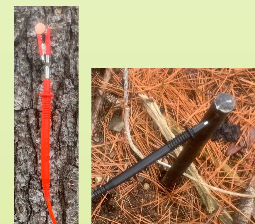
Close-up view of (+) and (-) tree voltage pins
