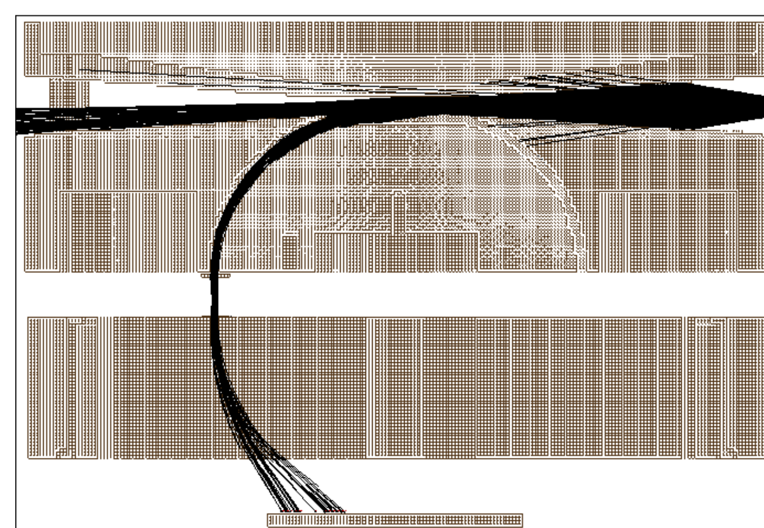
Figure 7. A SIMION simulation with particles accelerated to 800eV. Trajectories can be seen in black. The particles of the correct energy are deflected through the electrostatic analyzer. Between stage 1 and 2 they are accelerated to a higher energy. They are then separated by mass, with N_2^+ to the left and O^+ and to the right.
