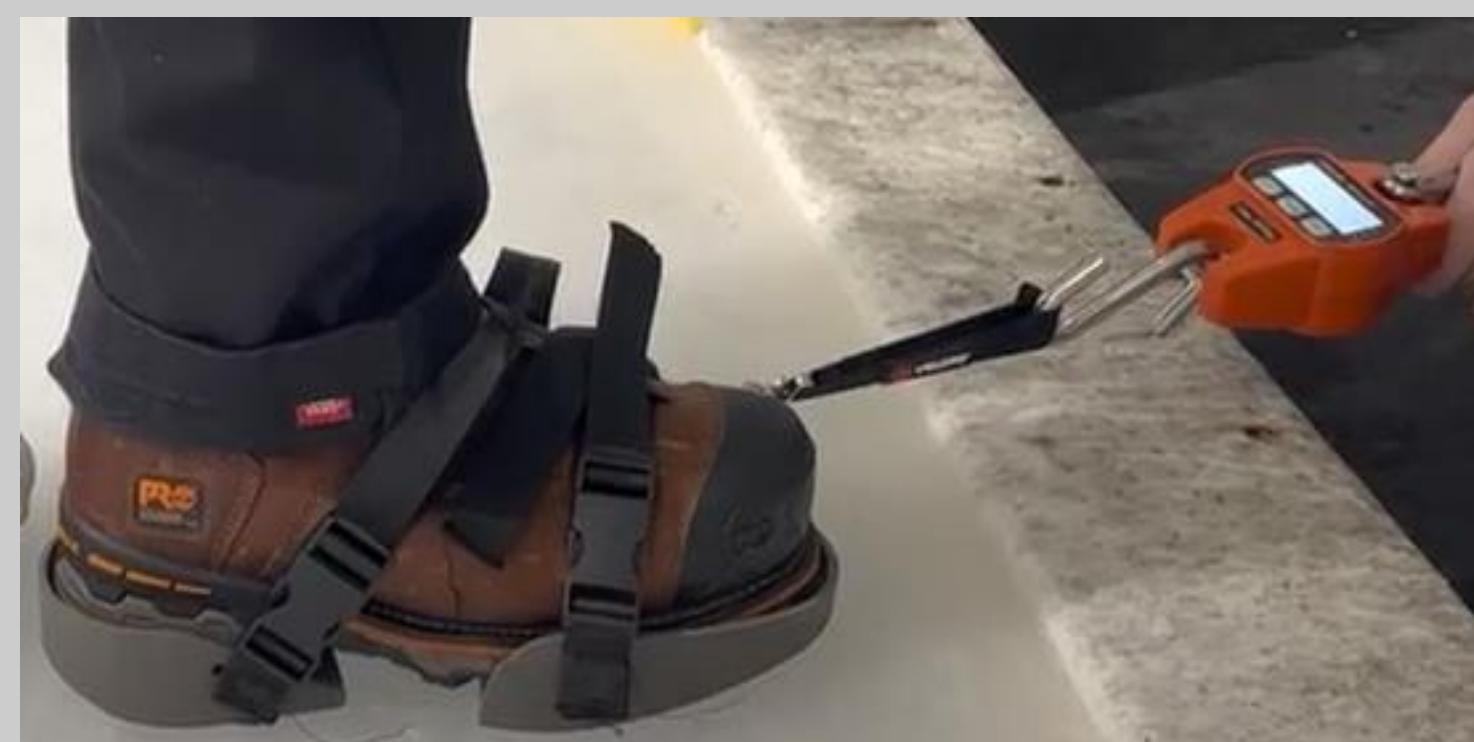
Setup of Friction testing (left): Crane scale used to measure force required for boot slippage
