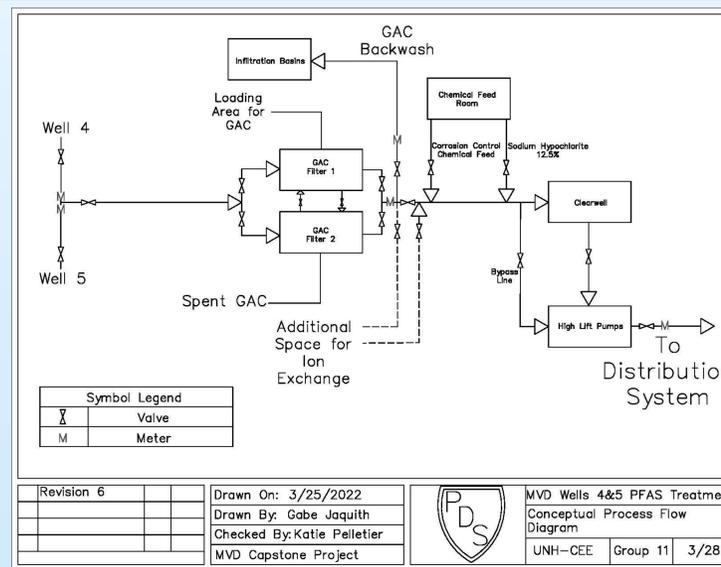
The flow diagram provides a basic overview of how the proposed treatment facility would operate. Through the diagram, we have illustrated the proposed treatment process and other key elements like backwashing and chemical feed.
