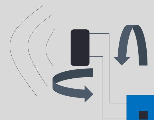
The sensor collects distance measurements as it spins
