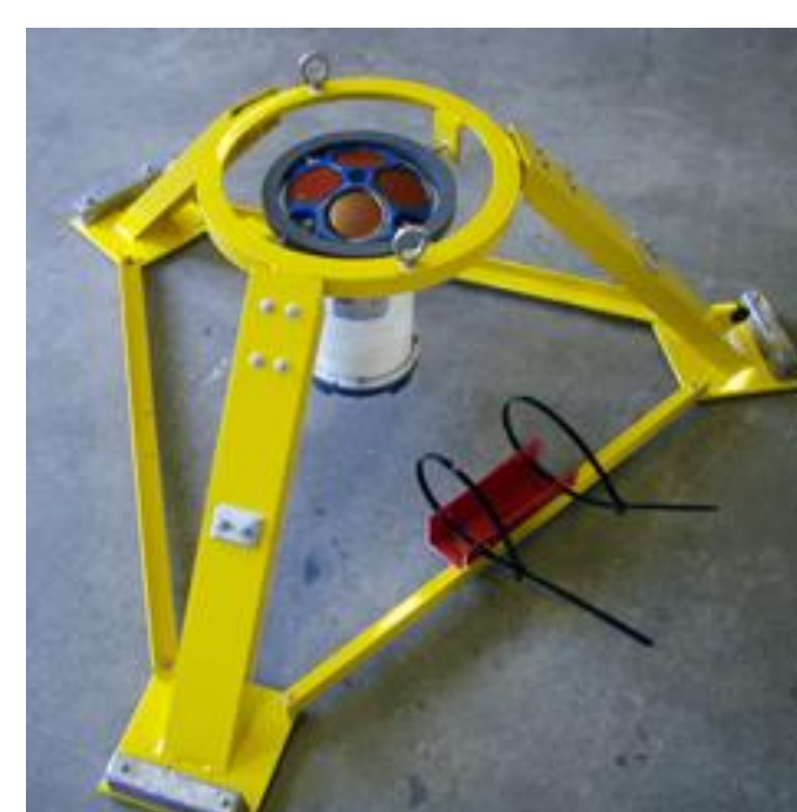
Figure 3. (Left) Acoustic Doppler Current Profiler (ADCP) mounted in a tripod. (Right) Lagged array of ADCPs that will be deployed in Hampton Inlet. Observations will be compared to the analytical solutions.
