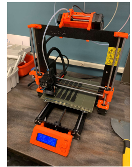
Figure 11: Prusa 3D printer in Olson Center printing tensile test specimens
