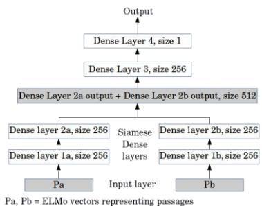
Siamese architecture used to model the similarity metric used for **UNH-dl**
